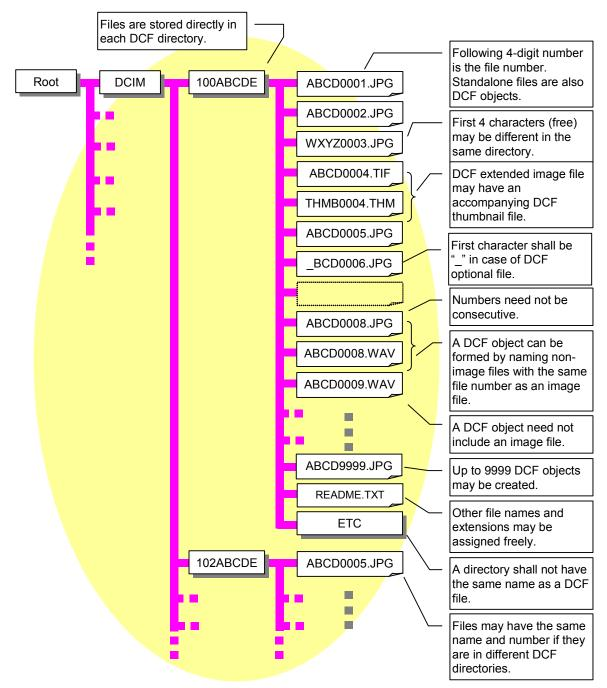
Figure 5 Typical file structure in a DCF directory
