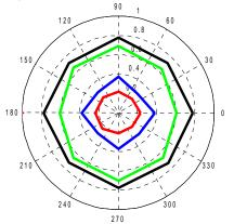
Figure 6: CFA-SLR modulation at 450 LP/PH.
