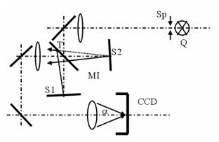
Figure 9 Diagram of the Michelson interferometer
