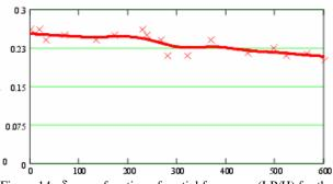
Figure 14:  $\delta_{RGB}$  as function of spatial frequency (LP/H) for the X3-SLR. The lack fall-off of color saturation with spatial frequency differs from other cameras tested.
