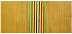
Figure 10: An example white-light interferogram from the Michelson interferometer. The fringe distance varies as a function of wavelength giving a color pattern useful for testing a camera's color resolution.
