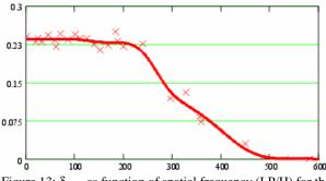
Figure 13:  $\delta_{RGB}$  as function of spatial frequency (LP/H) for the CFA-SLR. This loss of color at spatial frequencies above 300 LP/PH was typical of all digital cameras tested.
