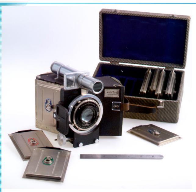
Devin Tri-Color has three plates with RGB filters and beamsplitting pellicles.
