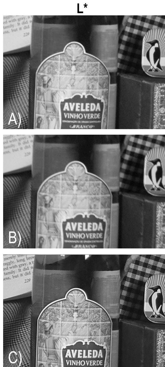
Figure 11. The luminance channel of images captured with a digital camera using A) a Bayer mosaic sensor, B) a Bayer mosaic sensor and a blur filter, and C) a Foveon X3 sensor that fully captures luminance information at every pixel location. Notice the artifacts caused by interpolation errors in A, softer lower resolution in B, and a clean sharp luminance record in C.
