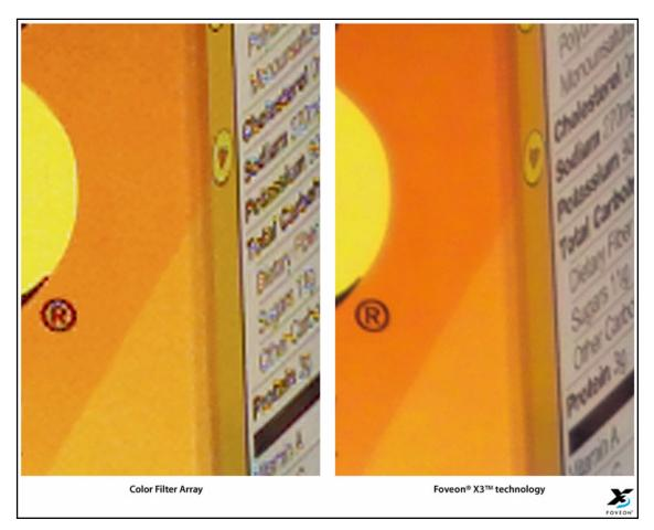
Figure 8 Image Quality Difference Between CFA and X3 – Color Accuracy
