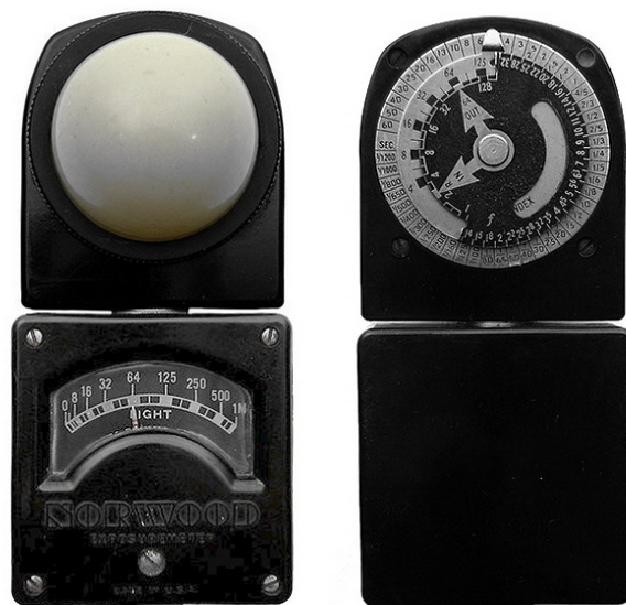
Figure 3. Norwood Director exposure meter ("Model A")
